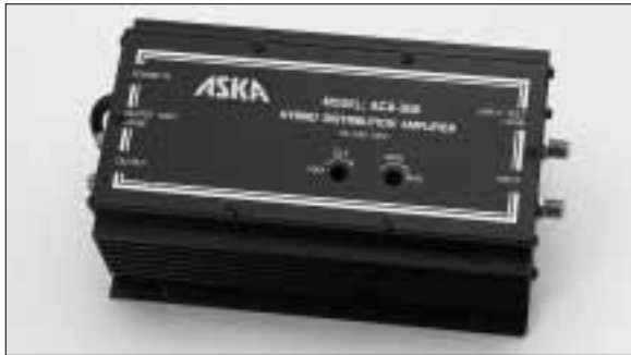
PUSH PULL CATV AMPLIFIERS With Tilt and Gain Control
