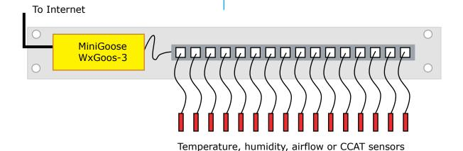
The remote temperature sensors can have an aggregate cable length of 600'. The connectors are RJ-12 receptacles. The MiniGoose is not included. A screwdriver is required to assemble the unit.
