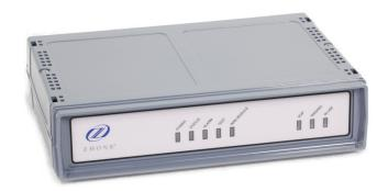
The zNID-GE-22xx series of indoor ONT's provide an ideal solution for FTTH deployments. The indoor ONTs are standards-based CPE designed for advanced triple-play deployments. The device provides for many features such as QoS, multicast video, and voice. The ONT is designed for high performance applications. The gigabit interface uses SFP's for the ultimate in flexibility. The SFP can be either copper or optical. A wide range of Gigabit SFPs are available which support distances from 10 to 60 km.
