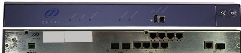
The zNID 97XX Series ONTs are designed to transport Gb data and T1/E1 circuit emulation services over a GPON or Active Ethernet optical link. Mobile backhaul applications are easily supported with 5 x GE ports and up to 4 x T1/E1 ports.
