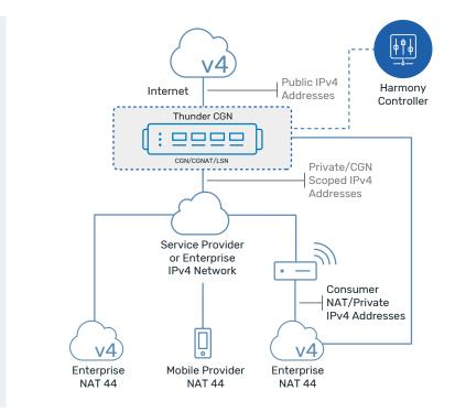
Use A10 Thunder CGN to leverage a standards-based mechanism-carriergrade network address translation (CGNAT), large-scale NAT (LSN), NAT444 or NAT44-to reclaim existing IPv4 space.
