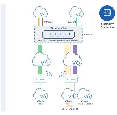
A10 Thunder CGN delivers IPv6 translation and encapsulation technologies, including prevalent protocol connectivity and interplay for phased IPv4-to-IPv6 transitions.
