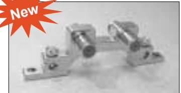
GB-3GD DUAL BLOCK Two 4 m/m holes and set screws for two separate ground wires 28dB Return Loss 5-2300 MHz
