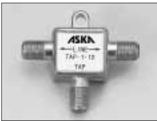
TAP-1( ) Freq. Range 5 - 1000MHz Available in dB value of 7, 12, 17, & 23dB Specify Tap value when Ordering
