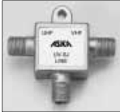
UV-SJ UHF/VHF BAND SEPARATOR/COMBINER VHF - 40-220MHz UHF - 470-890MHz
