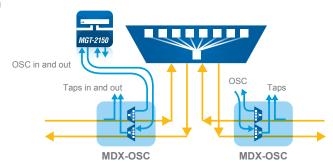
The MDX-OSC add/drop multiplexer includes two line-side monitoring ports for installation and testing.
