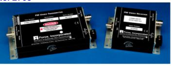
center frequency of 60 MHz to achieve this performance. While optimum performance is achieved with an RS-250C video input, the output level tracks the input level over the full optical loss range. Exceptional baseband bandwidth to beyond 15 MHz is typical, making the links usable for monochrome, NTSC color, PAL and HDTV applications.
