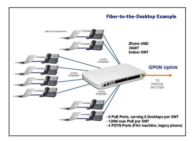
The 2600 Series GPON ONTs are ideally suited for Fiber-To-The-Desk applications where attached PoE devices can be powered directly from any or all of the ONT's four or eight PoE GE LAN ports simultaneously. Because up to four POTS ports are also available on the same ONT, legacy FAX machines, modems and analog phones can be conveniently connected.
