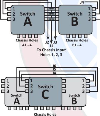
MUL-MS34-CH/K - Rack Mount Kit for three DP34s MUL-MS34-CH/A - Three DP34s Assembled in Chassis
