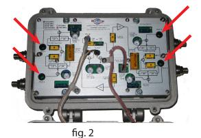
4. There are four holes that allow access to the four screws that tighten on the center conductor of the F-Connector. The holes are labeled, Port 1, Port 2, Port 3 and Port 4 (fig. 2)
