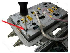
5. Using a Phillips-head screwdriver, tighten the set screws onto the F-Connector center conductors securely (fig. 3). Do not overtighten.
