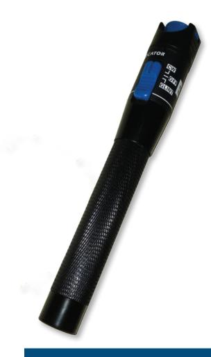
The 1, 10, 30 & 50 mW versions of the Multicom MUL-VFL is the easiest way to identify fibers from end to end and locate polished connector endfaces. The red laser shines through most yellow-jacketed fibers to help you precisely identify breaks, bends, faulty connectors, splices and other causes of signal loss. Reaching of up to 5 km\*, the MUL-VFL locates faults visually by creating a bright red glow at the exact location of the fault on both Singlemode or Multi-mode fibers.
