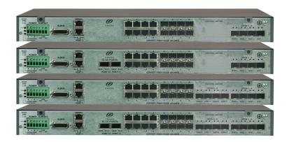
The Zhone MXK-190 provides next generation 1U GPON OLT features in a compact, hardened form-factor that makes it easy and cost-effective to deliver uncompromising triple play services throughout the serving area. Models are available with 4 or 8 GPON Ports. The ITU-T standard GPON technology provides 2.5Gbps downstream and 1.25 Gbps upstream bandwidth over a passive optical network on each of the 4 or 8 ports per unit.
