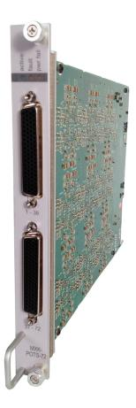
The integrated derived POTS lines convert packet voice to PSTN POTS allowing service providers to take advantage of a low-cost packet network and still provide subscribers with traditional POTS service. The card supports packet voice protocols SIP, MGCP, and H.248. For easy migration from TDM voice to packet voice, the MXK can be connected to the MALC Voice Gateway card to provide GR-303 or V5.2 termination with packet voice connection to the POTS card at a remote site.
