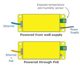
A self-contained climate monitor, the MicroGoose needs only an Ethernet connection and power. In a network with PoE, both are supplied through an Ethernet cable. Otherwise the included wall power supply is used.
