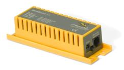
About the size of a candy bar, the MiniGoose II contains an internal temperature sensor, a digital sensor port and the same alert and monitoring functions as the WeatherGoose II.
