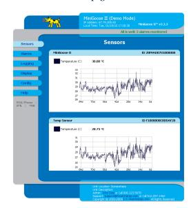
Sensor data and graphs are grouped by device, with internal sensors in the first box and remote sensors in the following boxes.
