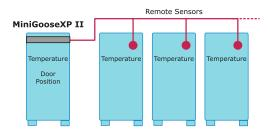
A single MiniGooseXP II wth remote digital sensors, can monitor up to 17 cabinets. The total aggregate cable length for digital sensors should not exceed 600'.
