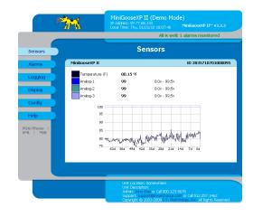
Readings from the internal temperature sensor and analog inputs are shown on the Sensors page.
