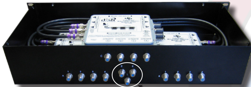
Rear of assembled unit with lid removed → Three Satellite Inputs
