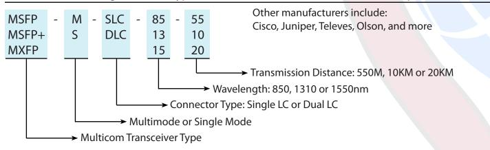
Example: MSFP-S-DLC-13-10 is a Single Mode, Dual LC Connector SFP with 1310nm wavelength going up to 10KM
