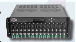
Power supplies, fans and management modules are hot swappable and are integrated into the chassis design leaving all 14 slots open for OTC modules. All OTC modules are plug in/hot swappable with RF inputs and outputs fixed to the chassis rear panel, simplifying module replacement.
