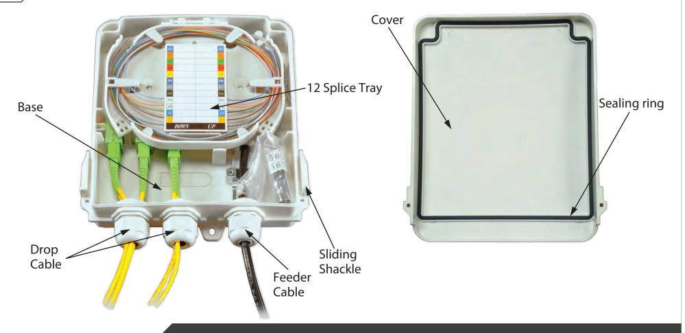
The FWP-8SC-12SP is one of a new family of plastic fiber wall mount boxes for fiber to the home. The box is light, compact, and designed to connect and protect your FTTH cables.
