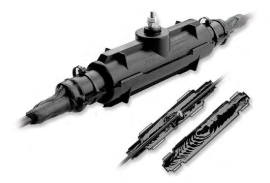
The Starfighter Mid-Span Grounding Closure is specifically designed to allow for meeting grounding and bonding specifications. The closure has a Gel Seal technology to provide for a water tight seal without the need for any additional grommets are special seals. The closure is also designed for re-sealing cable sheath damaged as a result of placing or outside plant events.
