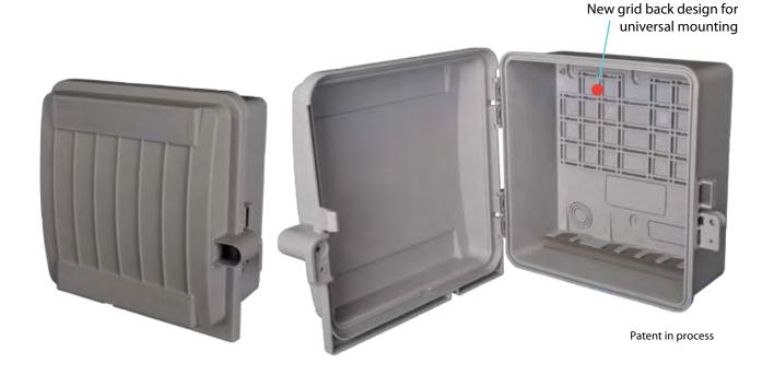
The RNI-1200 series enclosure is constructed with UV stabilized plastic, standard gray color. Removable door has dual locking systems and accepts custom logos/imprints. Cable entry points can be found on the bottom of this enclosure. Countersunk mounting holes for easy mounting on uneven surfaces. Back wall incorporated Flex-Mount arrangement, which incorporates mounting slots for greater flexability in mounting more products. Slots accept #6 & #8 screws.
