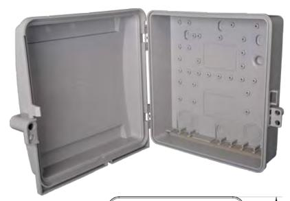
The RNI-1500 series enclosure is constructed with UV stabilized plastic, standard gray color. Removable door has dual locking systems and accepts custom logos/imprints. Cable entry points can be found on the bottom of this enclosure. Countersunk mounting holes for easy mounting on uneven surfaces.
