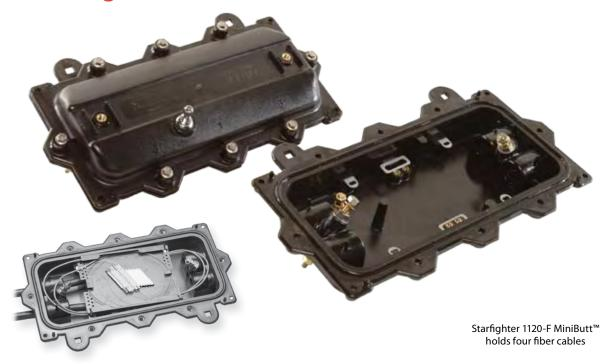
The 1120-F MiniButt Fiber Optic Splice Closure is designed for low count fiber splicing and in areas where space is a constraint. The closure incorporates an integrated gasket to prevent the ingress of water but to allow for ease in access.
