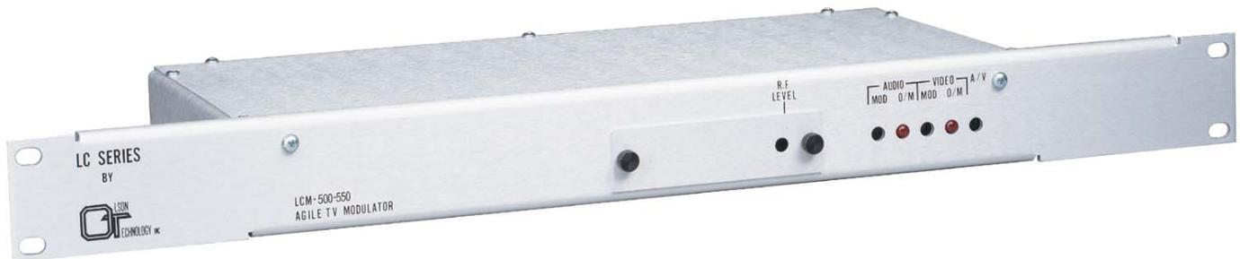
The **LCM-500-550** agile modulator series is a cost effective, SAW filtered unit that will fit most modulator applications. The **LCM-500-550** provides high level output on any channel from channel 2 (55.25MHz) to channel PPP (547.25MHz). Channels are selectable by front panel DIP switch and all F.C.C. offsets are tunable by front panel adjustment.
