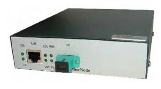
copper-to-singlemode optical fiber unmanaged media converter designed around the very latest ethernet transciever technology. It reliably transports full duplex 10/100 BaseT Ethernet from 0 to 60+ km on a single strand of fiber utilizing only one optical wavelength (i.e. 1310nm or one of eight CWDM ITU Grid wavelengths from 1490nm thru 1610nm).
