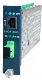
optical fiber unmanaged media converter 3RU module designed around the very latest ethernet transciever technology. It reliably transports full duplex 10/100 BaseT Ethernet from 0 to 60+ km on a single strand of fiber utilizing only one optical wavelength (i.e. 1310nm or one of eight CWDM ITU Grid wavelengths from 1490nm through 1610nm).
