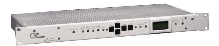
The **OTM-4870** has all the high end features required by the most sophisticated users of 100+ channels in cable televisions systems. Output frequencies may be selected by frequency in 12.5KHz increments or by channel designation. EIA or OLSON channel plans can be selected for standard channel, HRC or IRC assignments.
