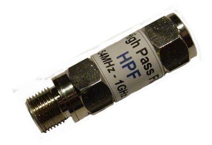
This new High Pass Filter has been designed for indoor/outdoor use. Each unit has been tested to 10psi (water test), The female contacts (F61) have a neoprene insert with a 360 degree contact which provides a high holding force. The male connector has an integrated "O Ring"
