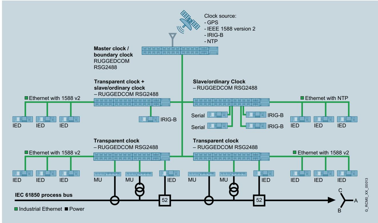
The RUGGEDCOM RSG2488 provides all IEEE 1588 clock modes required to support a complete precision timing protocol solution for IEC 61850 based substation automation.
