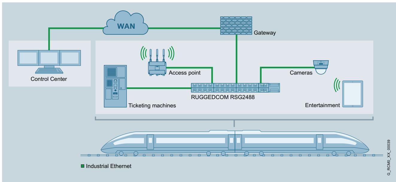
Onboard communication with high density, full Gigabit Ethernet, using the RUGGEDCOM RSG2488 with M12 Gigabit modules.
