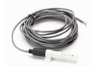
Each of the two varieties of the sensor is housed in a 4 inch Delrin plastic tube with ventilation holes. The nylon clamp permits the sensor to be screwed to a metal or wood surface. Cable lengths of 20 and 100 feet are available.
