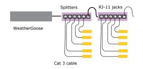
Telephone-type splitter blocks permit up to 16 RTAFH sensors to attach to the WeatherGoose series of climate monitors. Punch-down blocks can also be used to connect the Cat 3 wires.
