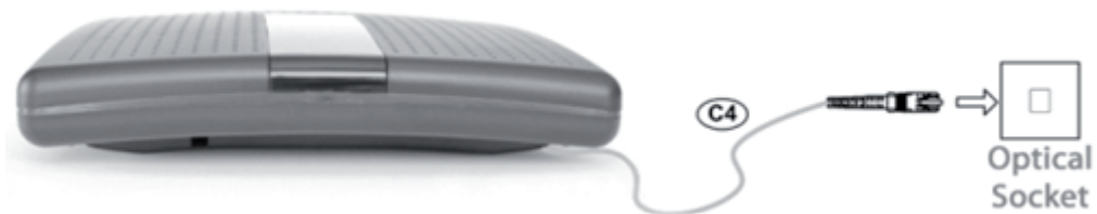
Figure 4-15: ONT 769503-SFU interfaces connection 1 (PON Interface)
