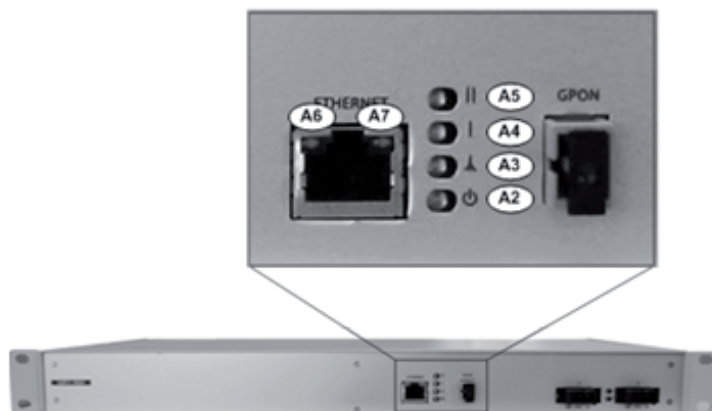
Figure 6-32: ONT 769503-MBH status LEDs
