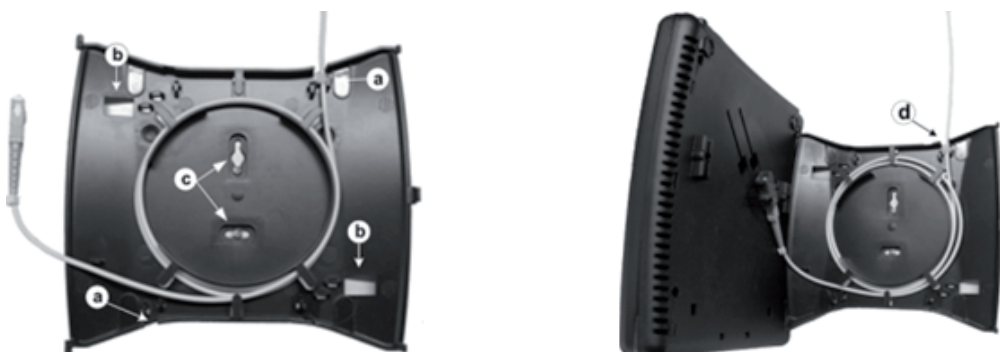
Figure 4-12: Optical cable installation –wall mount
