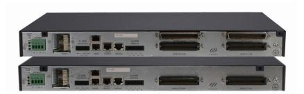
The Zhone MX-150 provides next generation IP DSLAM features in a compact, hardened form-factor that makes it easy and cost-effective to deliver uncompromised triple play services throughout serving area. Models are available with 48 ADSL2 + Ports with option of integrated POTS splitters.
